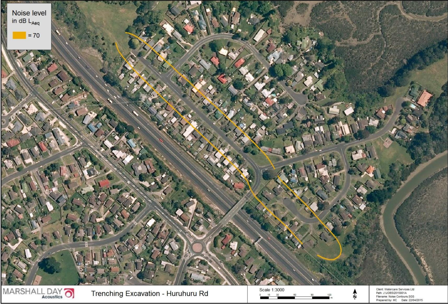
Figure I3: Huruhuru Rd Trenching
